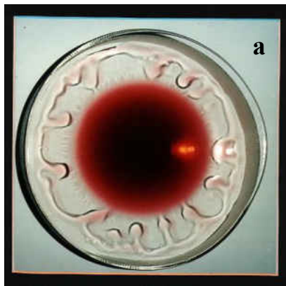
Figure 1 a) Top view of wine glass and wine tears (chemical variation of surface tension) 1 b) Vapor bubbles move toward hotter region in the center of the heater wire (thermal variation of surface tension) 2
